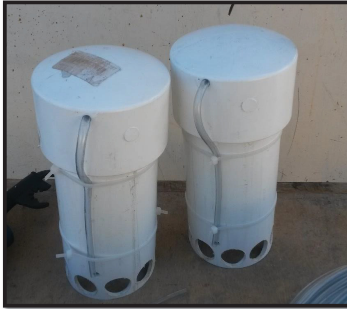
Figure 10. Bell siphon with rubber tubing to be places over standpipes
