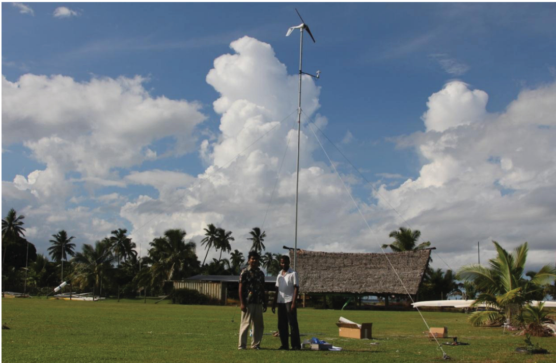
Fig. 6.3 Setup for testing of the Air X wind turbine at the Marine campus
