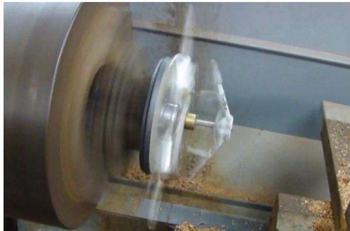
Fig. 5.25 Governor arms actuated at 883rpm. Partial engagement occurs at 635rpm, whereas full engagement occurs at 1000+rpm
