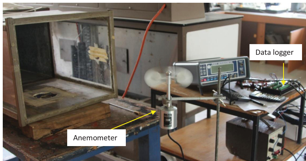
Fig. 6.9 Setup for anemometer for direct velocity measurement
