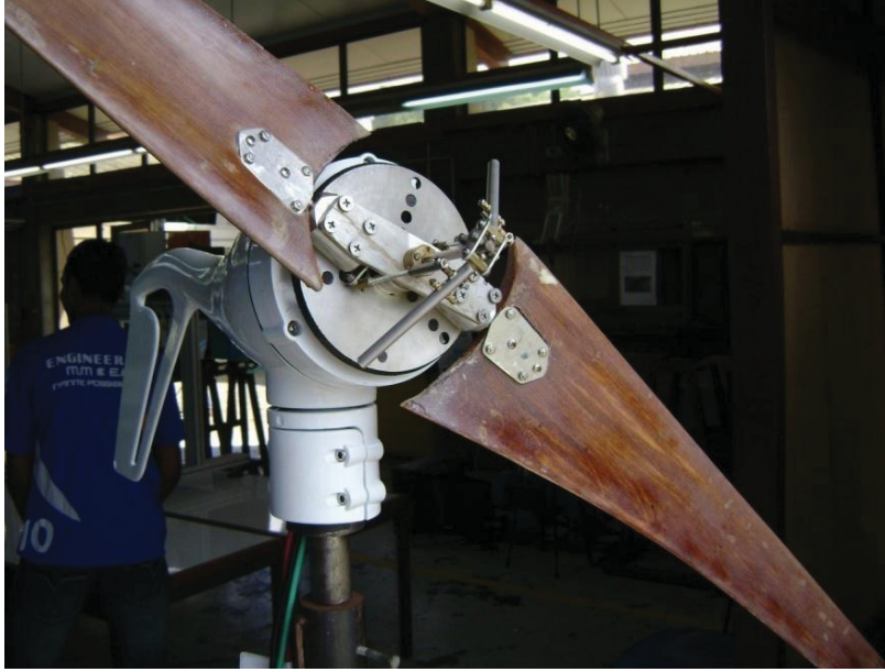
Fig. 5.21 Fabricated fiber coated wooden 2-bladed rotor fitted on an Air X Marine 400Watts wind turbine
