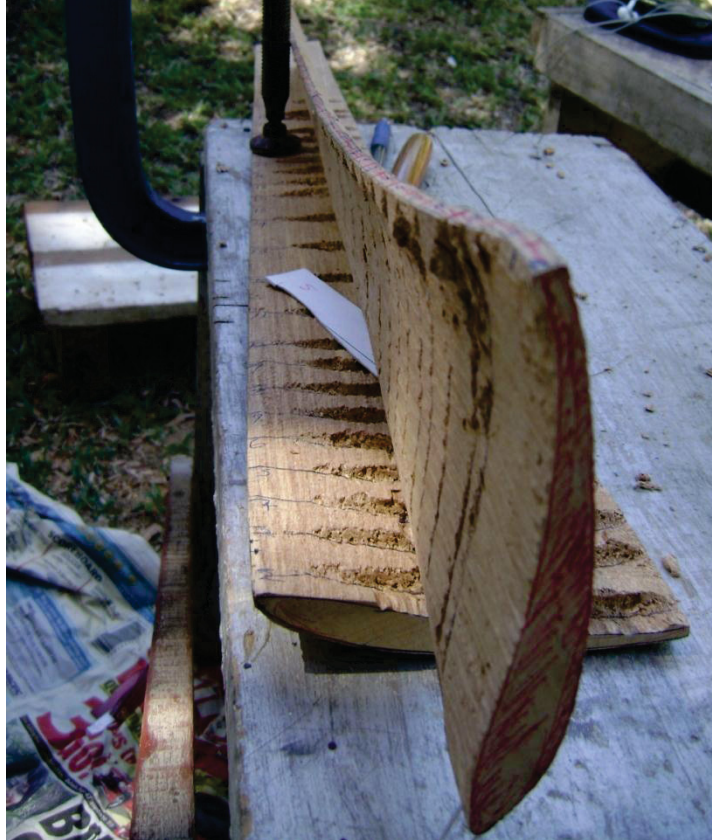
Fig. 5.19 Roughly completed blade with the twist clearly visible on the trailing edge of the blade
