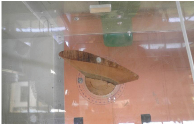
Fig. 4.5 Airfoil inserted in test section for measuring lower surface pressure distribution
