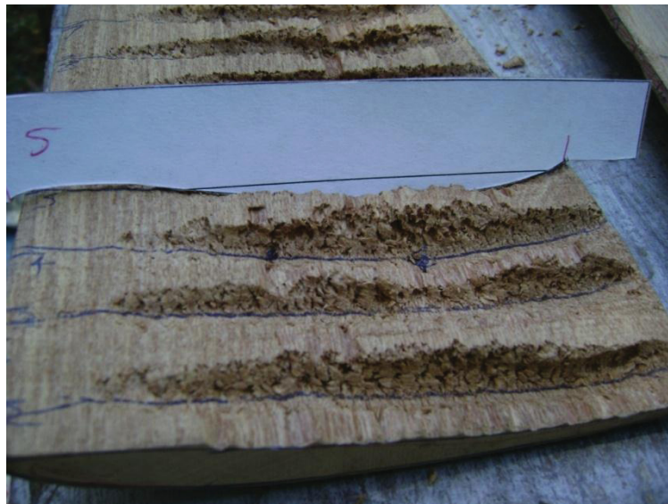
Fig. 5.18 Templates being used to carve the airfoil profile together with the twist distribution onto the bottom side of the blade
