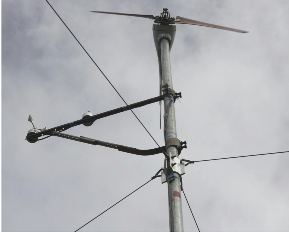
Fig. 6.4 Close-up view of the Air X turbine with the new 2-bladed rotor and anemometer setup
