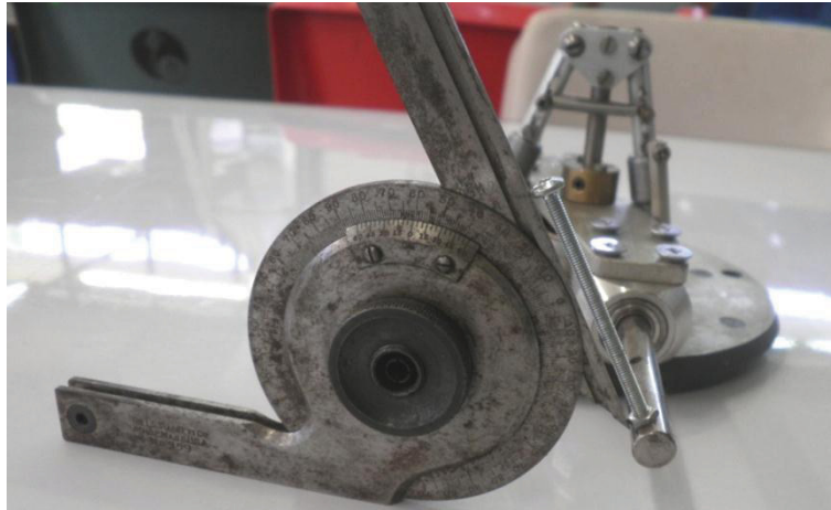
Fig. 6.12 A vernier protector being used to set the pitch angle, \beta at the root on each blade shaft
