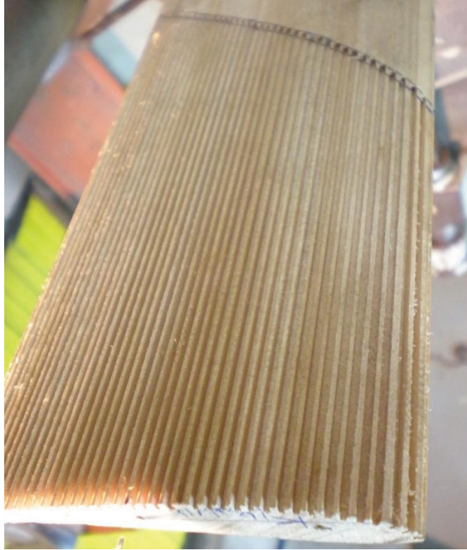
Fig. 4.3 Details of groves cut into the upper surface of the airfoil for pressure tubes
