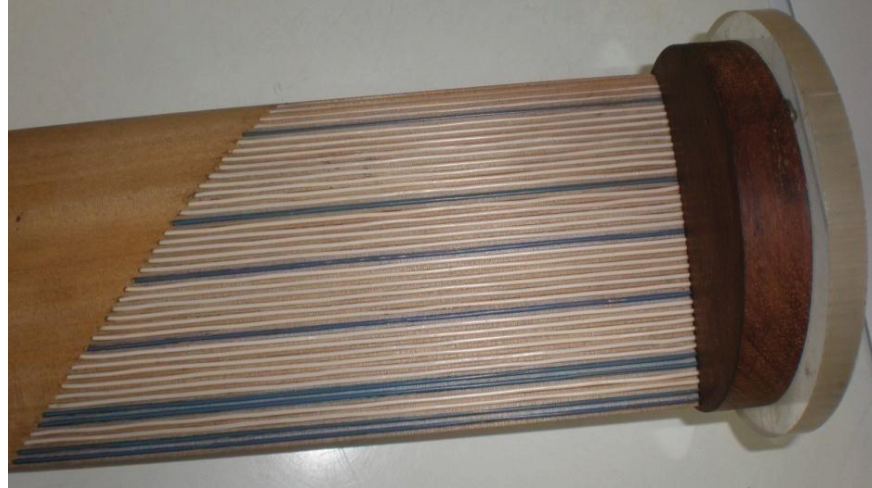
Fig. 4.4 Finished airfoil ready for upper surface pressure measurements
