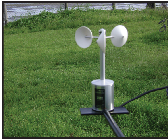
Figure 2.9 Pulse output A101M anemometer used for wind speed monitoring at Laucala Bay and Nabua sites.
