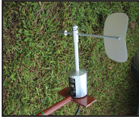
Figure 2.10 Potentiometer wind vane (low torque) W200P/L used for wind direction monitoring at the Nabua and Laucala Bay sites.
